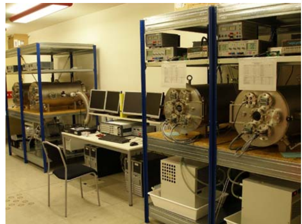
Figure 5. PHM QM Lifetime test bench
